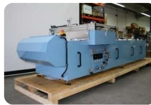
Project: AIRBUS Bremen, 12 x 4 m Infrared Dryer for curing of Aircraft Tails
